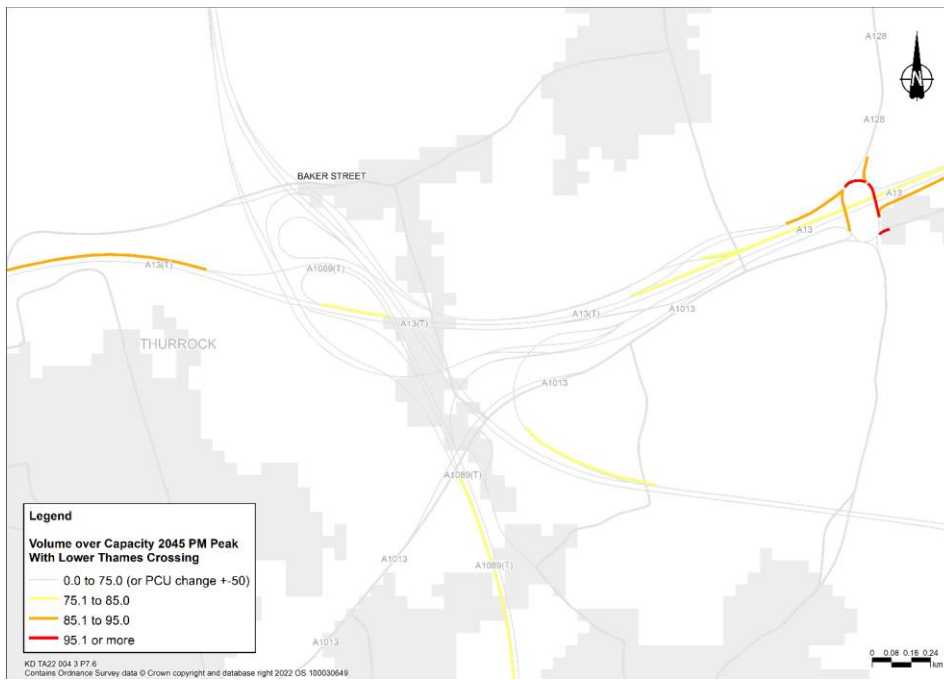
Plate 7.6 Volume to capacity at the A13/A1089/A122 Lower Thames Crossing junction – PM peak 2045
